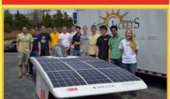
4.80m x 1.80m x 1.22m 1000W Suniva Mono-Si 7.5kW NGM SCM150 4130 Steel Space Frame Three 14" NGM AI Rims
