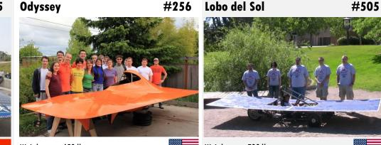
450 lbs Weight: Batteries: Trustfire Li-Ion Chassis: Titanium Motor: NGM SC-M100
