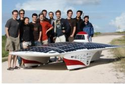
Weight: 414 lbs Solar Cells: Sunpower C50 Batteries: WANMA Li-Po Carbon Monocoque Chassis: Motor: NGM SCM-150
