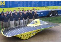
Weight: 700 lbs Solar Cells: Emcore ATJ/BTJ A123 Lithium Ion Phosphate Batteries: Chassis: Carbon Fiber CSIRO Motor:
