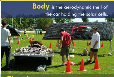
Chassis is the structural frame of the car forming the driver cockpit.
