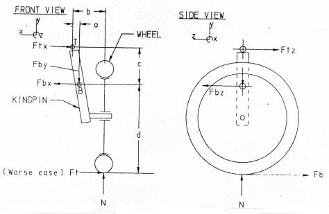
For static conditions, with an equal weight distribution on 4 wheels, N=W/4. If a 25% weight shift to the front wheels is assumed during braking, N=1.25\*W/4 on each front wheel.
