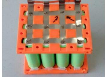
well with Spot Welded Nickel buss by the team after some spot weld development.
