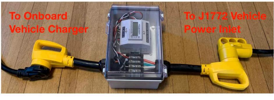
The kWh hour meter is watertight, weighs 6lb, and has enclosure dimensions of 11" L x 7.5" W x 4.5" H with a connector to connector length of 27".
