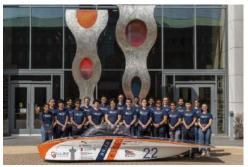
L x W x H: 5.00m x 1.20m x 1.00m Weight: 192kg Array: 1000W SunPower Silicon Batteries: 5.2kWh Li-lon (20kg) Motor: 1 Mitsuba Wheels: 4 GH Craft Carbon Fiber 16" Chassis: Semi-Monocoque Carbon Fiber Panel
