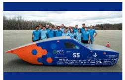
L x W x H: 4.90m x 1.85m x 1.25m Weight: 330kg Array: 1271W SunPower Maxeon Silicon Batteries: 9.2kWh Li-lon (46.6kg) Motor: 2 Mitsuba M2096D-III Wheels: 4 Carbon Fiber 16" **Chassis:** Composite Material Sandwich Panels
