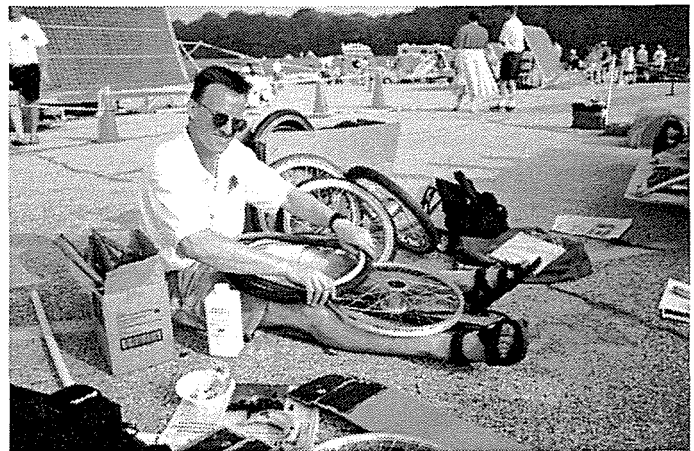
Figure 6.8.3: Inferior components do not equal inferior performance. University of Minnesota used standard bicycle wheels and tires, but experienced only two flat tires. Minnesota completed all 1246 miles and regularly saw speeds in excess of 50 mph. David Craig carefully installs an inner tube using baby powder to keep away dirt and to prevent pinched tubes. Also, notice the heavy-duty rim strips to prevent spoke punctures.
