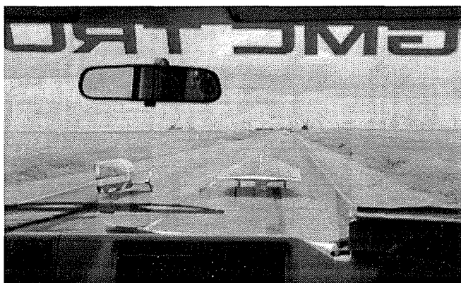
Figure 6.5.6: The TNE-3 from Northern Essex Community College passes MIT's Manta on one of many long stretches of highway on the Sunrayce 95 route. Notice that if the TNE-3 body were unwrapped, its surface area would be about the same as just the top-side surface area of the MIT car.
