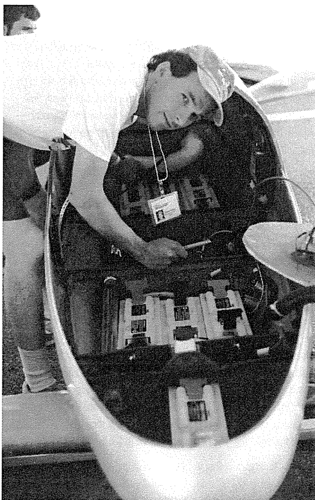
Figure 6.4.3: Northern Essex Community College co-captain James Nelson checks the Delphi battery pack positioned at the base of the vehicle. The driver was isolated by a Kevlar battery enclosure and seat.
