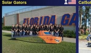
225kg • 5.00m x 1.00m x 1.50m 960W Mono-Silicon Sunpower Solar Array
