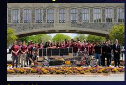
254kg • 4.50m x 1.80m x 1.20m 950W Mono-Silicon Sunpower Solar Array 19.9kg 4.7kWh Lithium Ion LG Batteries 1 Aegean Dynamics Motor 4130 Steel Tube Chassis 4 Aluminum Wheels • Bridgestone Tires
