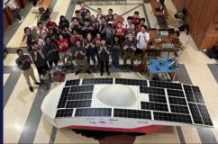
226kg • 4.95m x 1.02m x 1.25m 945W Mono-Silicon Sunpower Solar Array 35.5kg 4.9kWh LiFePO4 K2 Batteries 1 Mitsuba Motor Carbon Fiber Sandwich Panels
