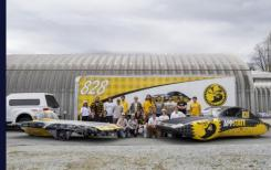
500kg • 4.74m x 2.10m x 1.24m • 2 Seats 1212W Mono-Silicon Sunpower Solar Array 122kg 13.8kWh Lithium Ion Envision Batteries 2 Mitsuba M2096-D3 Motors Carbon/Kevlar Honeycomb Sandwich Panel 4 Custom Aluminum Wheels • Bridgestone Tires
